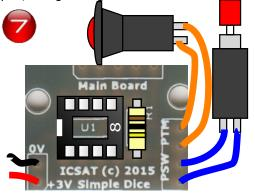
Carefully insert the PIC chip with the notch matching the notch on the DIL socket.
